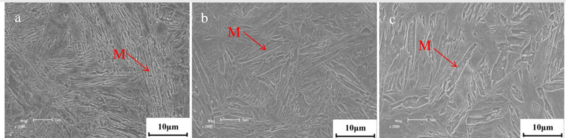
SEM micrographs showing the microstructures of steels after HS-DP process for (a) Salt bath + water quenching; (b) salt bath + oil quenching; (c) salt bath + air cooling
